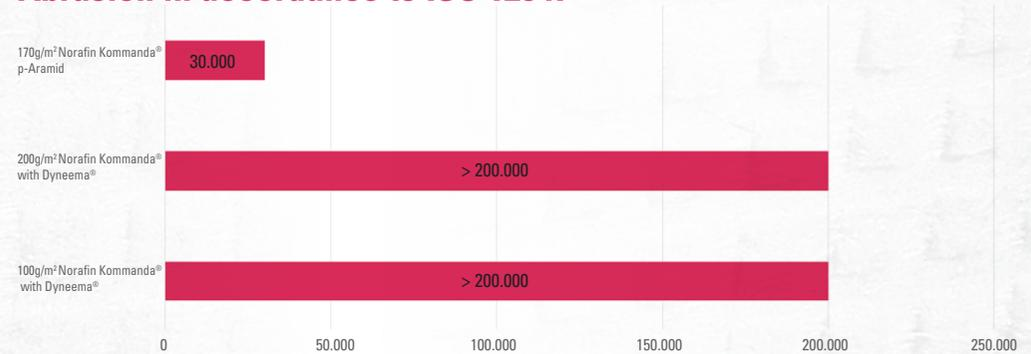
The Martindale-Method simulates natural wear, where the textile sample is rubbed against a standard abrasive surface with a specified force. The results of more than 200.000 cycles for Norafin Komanda® with Dyneema® show good mechanical stability and high strength of the nonwoven product during the life-cycle in a ballistic vest.
