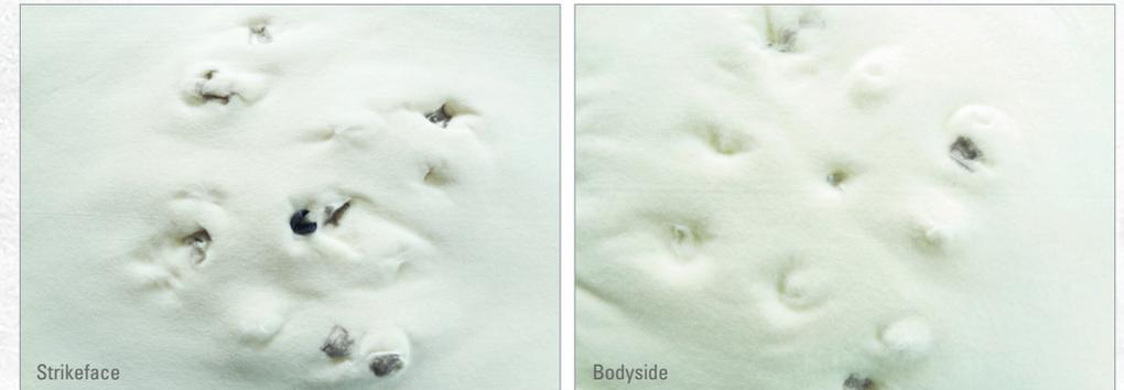
**Strikeface:** During the shooting the nonwoven is catching the fragments efficiently due to the high strength in combination with high flexibility and density.
